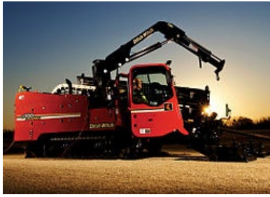
A directional boring unit in action.
